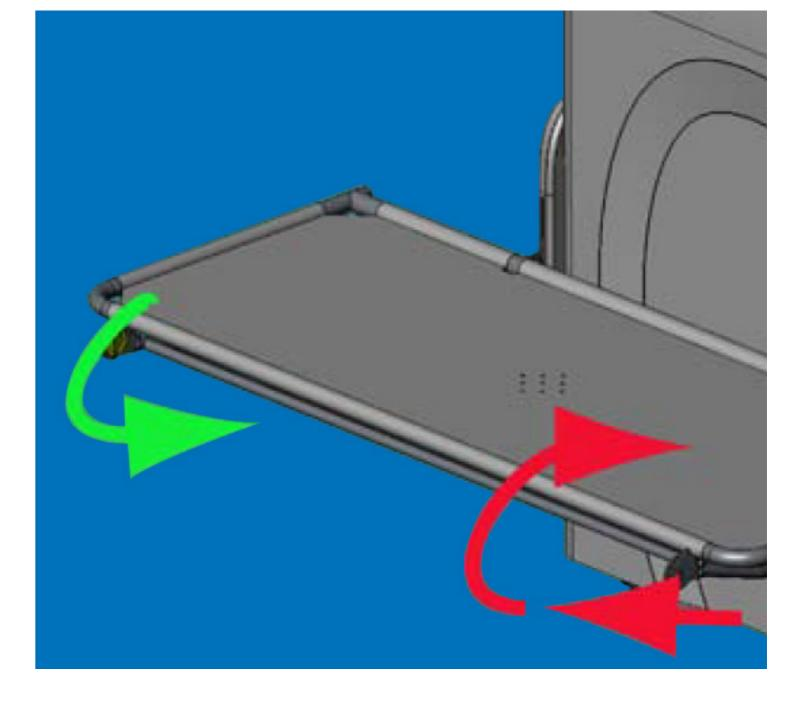
It will then lock under the bed. To replace the guard lift it slightly towards you, it will release, rotate upright and drop into position.
