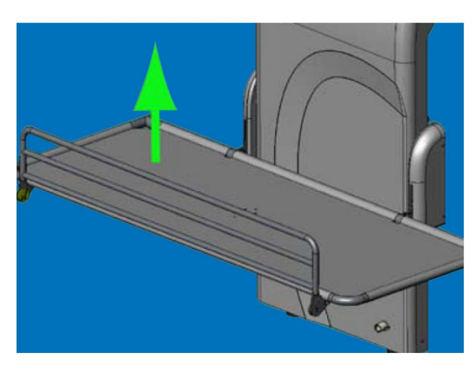
Operating the guard. Folding the guard. Lift the guard upwards.
